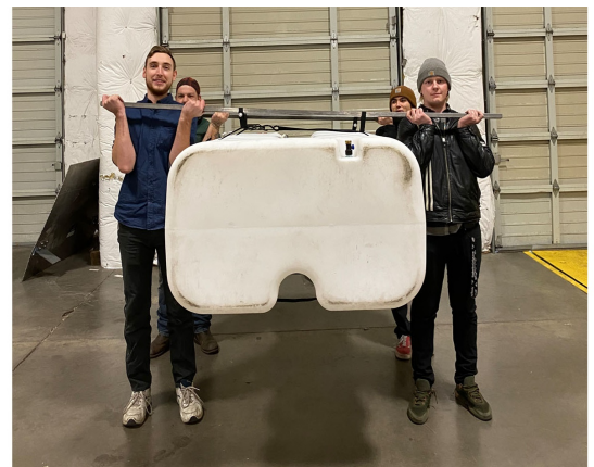
Lifting the unit via pipe or 2x4 through the handle loops
